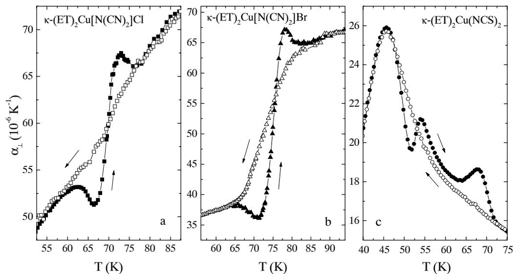
Fig. 2: Blow-up of the cross-plane thermal expansion coefficient around the glass-like transition(s) at  $T_g$  for various  $\kappa$ -( $ET$ ) $_2X$  salts. Arrows indicate cooling and heating runs.
