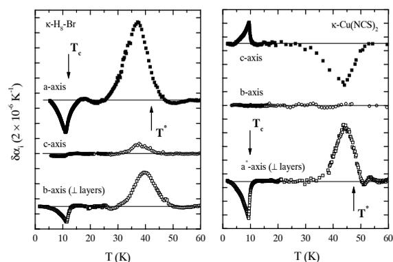
Fig. 3: Anomalous contributions to the uniaxial thermal expansion coefficients at  $T_c$  and  $T^*$  derived by subtracting a smooth background contribution.
