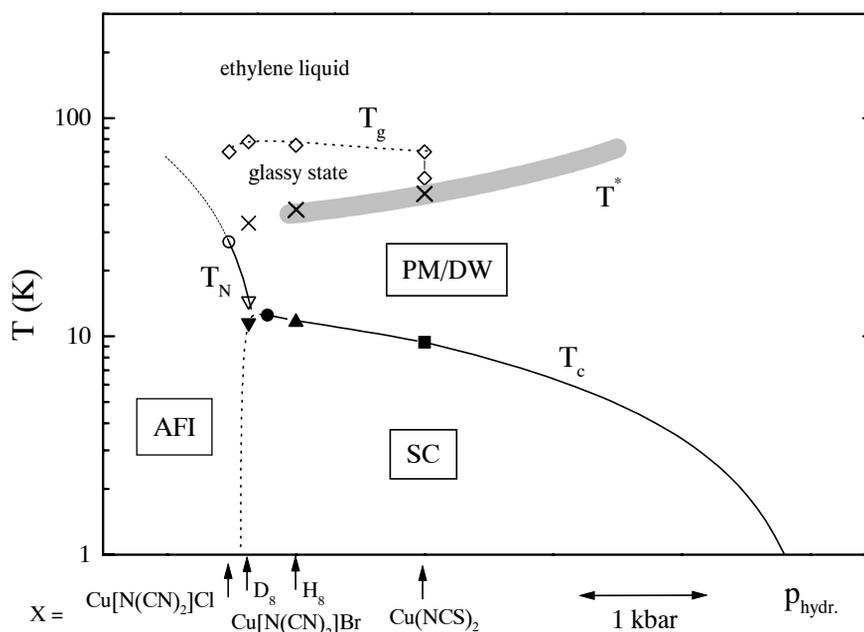
Fig. 5: Compilation of thermal expansion anomalies for the various  $\kappa\text{-(ET)}_2\text{X}$  salts in a pressure-temperature phase diagram. Arrows indicate the location of the different salts at ambient pressure. AFI, PM/DW and SC denotes antiferromagnetic insulator, paramagnetic metal in coexistence with a density-wave state and superconductor, respectively. Solid lines represent the hydrostatic pressure dependences of  $T_N$  and  $T_c$  taken from the literature.
